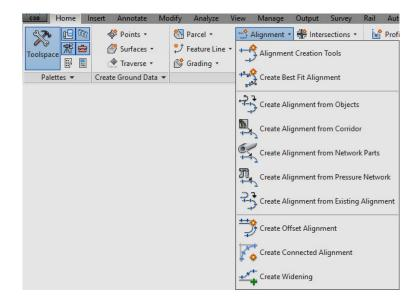
Alignment Creation Tools gives you the constrained based design options. Constrained based design will maintain tangency based on 3 choices:
