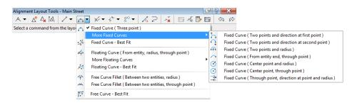
2. Floating Curve – Maintain tangency at the start, while one end is not connected to another object. For example, curves off the end of a line.
