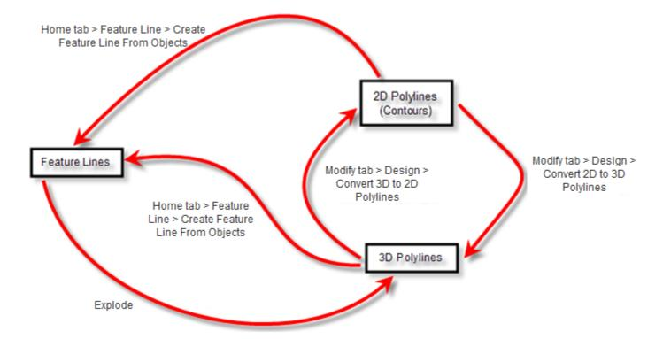
The figure below explains the general workflow when adding data to a surface when using the grading tools.
