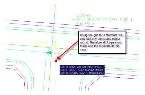
b. Profile View – You can hot grip the invert, centerline, or crown of a pipe. You can also multi-hot-grip grips by holding down shift while selecting the grip.
