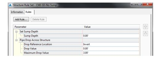
This next step is to either draw the pipe run or convert a polyline to a pipe network. You should make a note to realize that structures and pipes can only be connected together if they are in the same pipe network. Therefore you can start with one polyline, but then you need to edit the network in order to add more objects to the pipe network.
