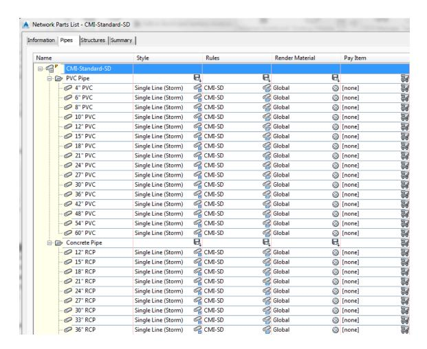
3. Right-click an example rule set, and then select edit. For both pipes and structures. See the manual for a detailed explanation of each rule.
