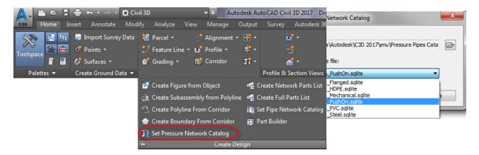
Set the catalog to the desired material, and then create a new parts list for that material. For example, PVC contains a fire hydrant, while the others do not.
