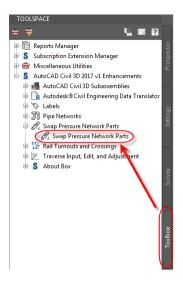
b. In Civil 3D 2018/2019, the user can swap the parts directly from the edit ribbon tab for pressure networks.
