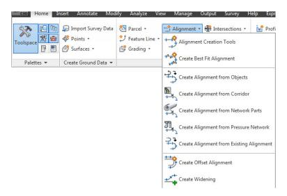
Alignment Creation Tools gives you the constrained based design options. Constrained based design will maintain tangency based on 3 choices:
