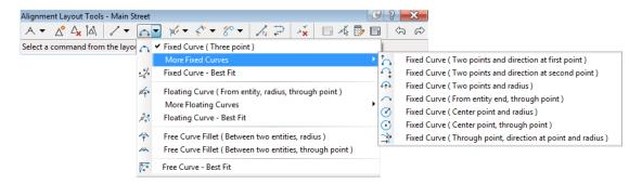
2. Floating Curve – Maintain tangency at the start, while one end is not connected to another object. For example, curves off the end of a line.
